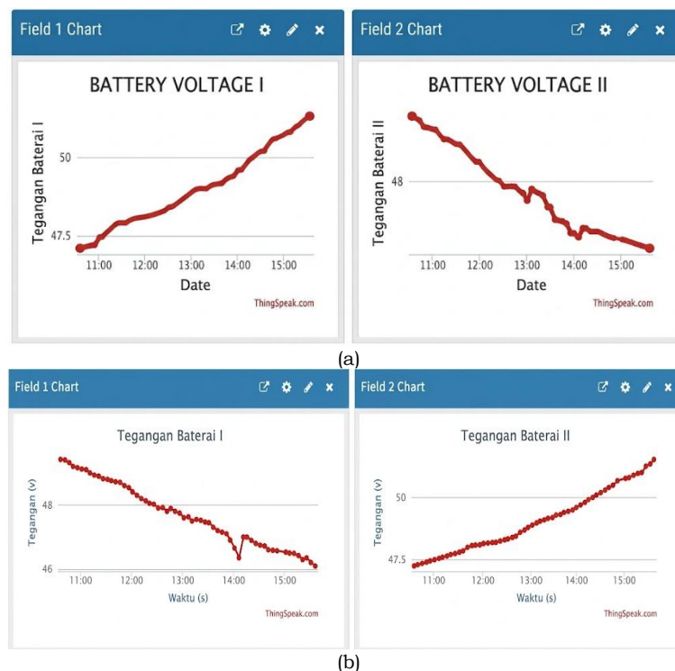
Figure 7. Monitoring data and battery voltage measurement results.
