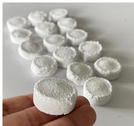
Figure 5. HAp/chitosan/PVA scaffold fabricated using the freeze-drying method.
