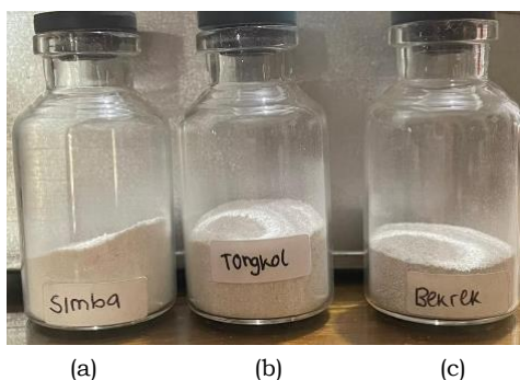
Figure 1. Furnace results of (a) simba fish, (b) mackerel tuna, and (c) bekre fish bones
